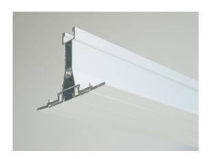
**TripleAir 55mm** T-bar extrusion profiles and joints have an identical geometry, allowing for a tight connection and preventing uncontrolled particle deposition during installation. Cruciform joints have penetrations suitable for cables, sprinklers or a closed insert. Tee joints and corners are available as casting without penetration.
