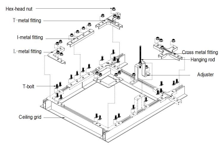
The HD Grid can accommodate fixings and hangars—room side. By simply removing the central cover, hangars and fixings can be fitted to support other services within the room.
