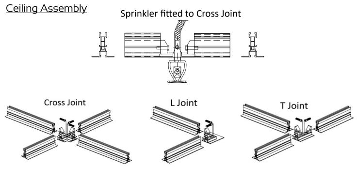
The HD Grid can accommodate fixings and hangars—room side. By simply removing the central cover to reveal a sliding track to which hangars and fixings can be fitted to support other services within the room.
