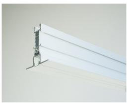
**TripleAir 55mm** T-bar extrusion profiles and joints have an identical geometry, allowing for a tight connection and preventing uncontrolled particle deposition during installation. Cruciform joints have penetrations suitable for cables, sprinklers or a closed insert. Tee joints and corners are available as casting without penetration.
