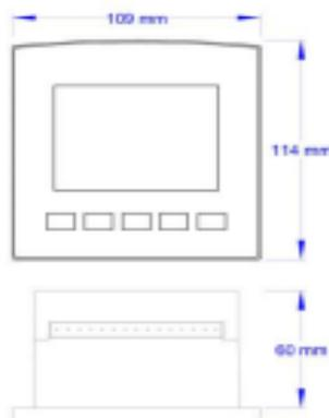
The ACF controller is an off the shelf controller which can be programmed individually to control collate and display the fan details on screen. Each unit can be tailored to customers specific requirements.
